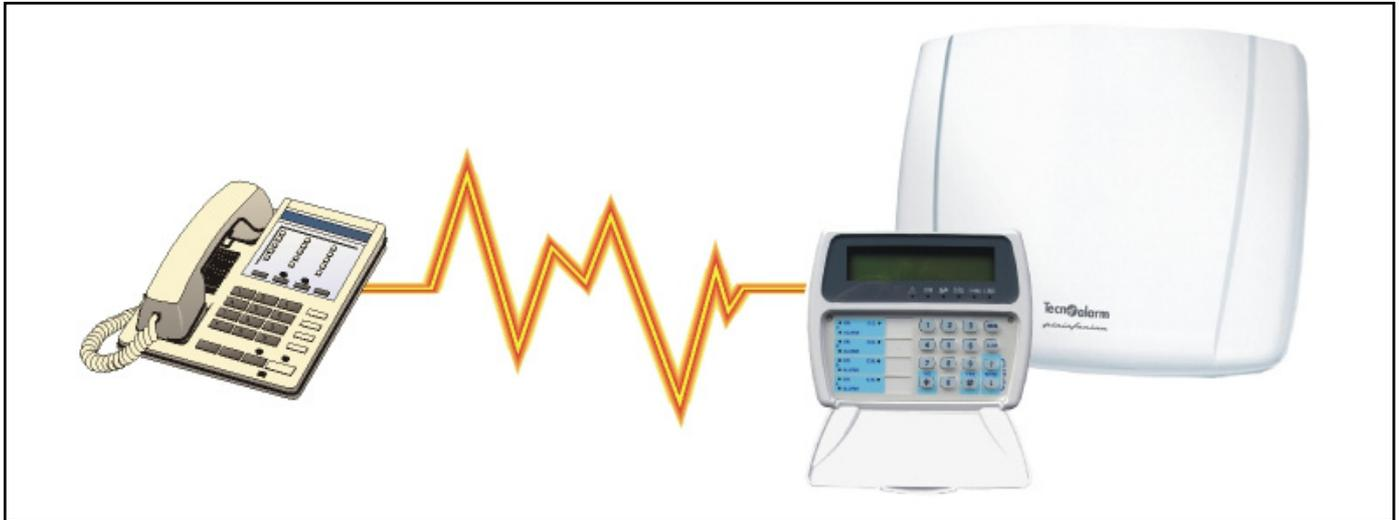
The telephone menu permits system status check and the initiation of a number of operations (telephone menu) calling the control panel on purpose, whereas it permits the verification of the alarms (RDV<sup>®</sup>) during a vocal alarm call received.
