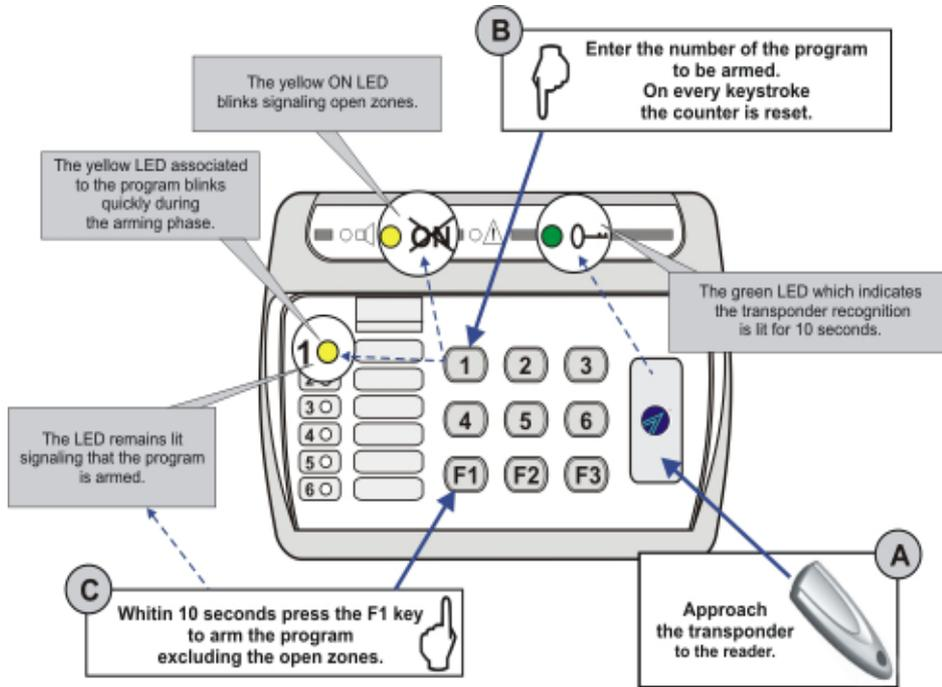
**A -** Approach the transponder to the reader (the green transponder LED is lit).
