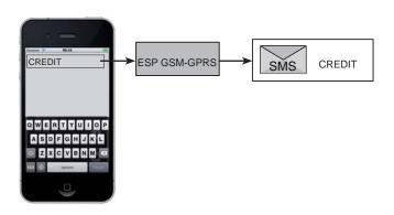
If the internal GSM interface ESP GSM-GPRS and/ or the external GSM transmitter TECNOCELL use the prepaid SIM cards, it is necessary to periodically check the remaining airtime.
