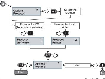
Press 2 to select the submenu, and press YES to confirm. The submenu permits configuration of the connection port PROG INTERFACE with the communication protocol for a computer (Tecnoalarm software) or a local printer. Select the protocol using the numerical keys.
