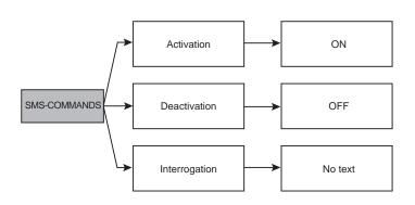
The user can activate/deactivate the remote controls and check the status by means of the SMS-COMMANDS. Activation - The command to activate the remote control is ON.
