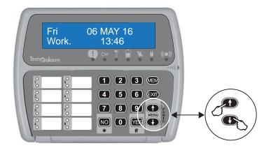
To release a panic alarm, press the arrow up and down keys simultaneously.
