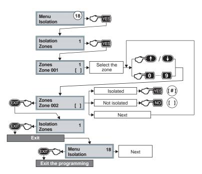
Select the Insulation menu, and press YES to confirm. Select the zone to be isolated using either the arrow keys or the numerical ones.
